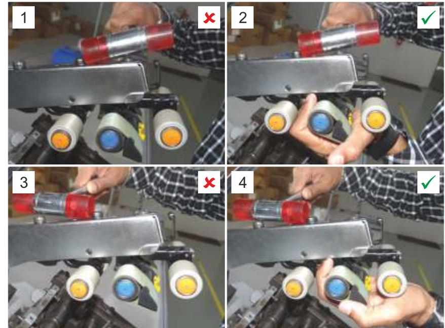
Image 1: While pushing the middle top roller back, do not tap the middle weighting element fixing screw without providing any support
